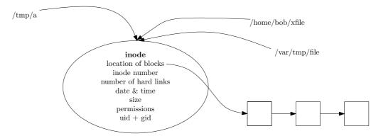
This inode contains several meta information and the location of that file on the disk (that part of the picture does absolutely not reflect the real situation).
