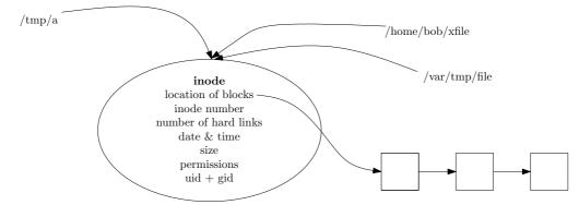
This inode contains several meta information and the location of that file on the disk (that part of the picture does absolutely not reflect the real situation).
