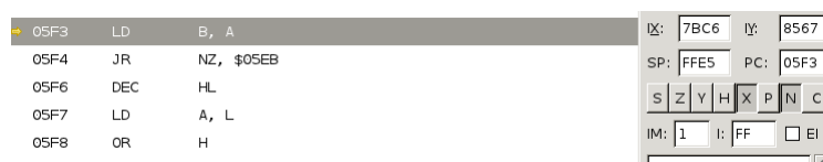
Figure 4.37: The value of PC is 05F3 as the address of the current instruction
